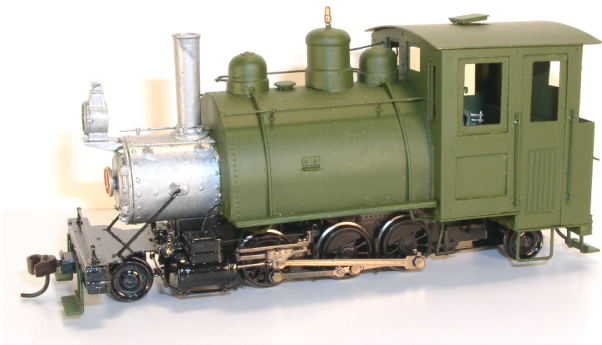
Major subassemblies mounted on chassis.
